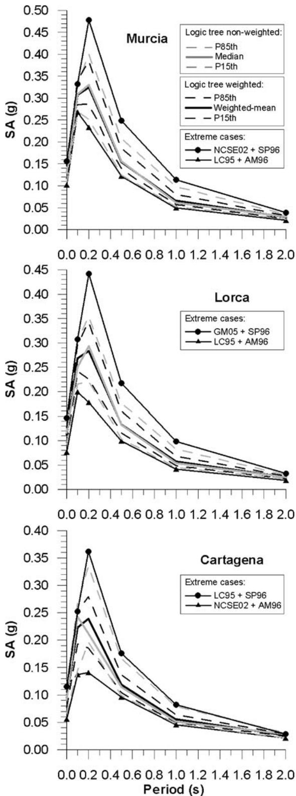
◀ **Fig. 9** Comparison among the resulting UHS from non-weighted and weighted solutions of the logic tree at Murcia, Lorca and Cartagena. Maximum and minimum spectra arising from specific choices of seismic source zonings and ground motion attenuation models (extreme cases) are also shown at each city
