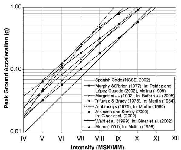
**Fig. 1** Comparison among different intensity-to-PGA conversion equations used in previous seismic hazard studies of the Province of Murcia or areas enclosing it
